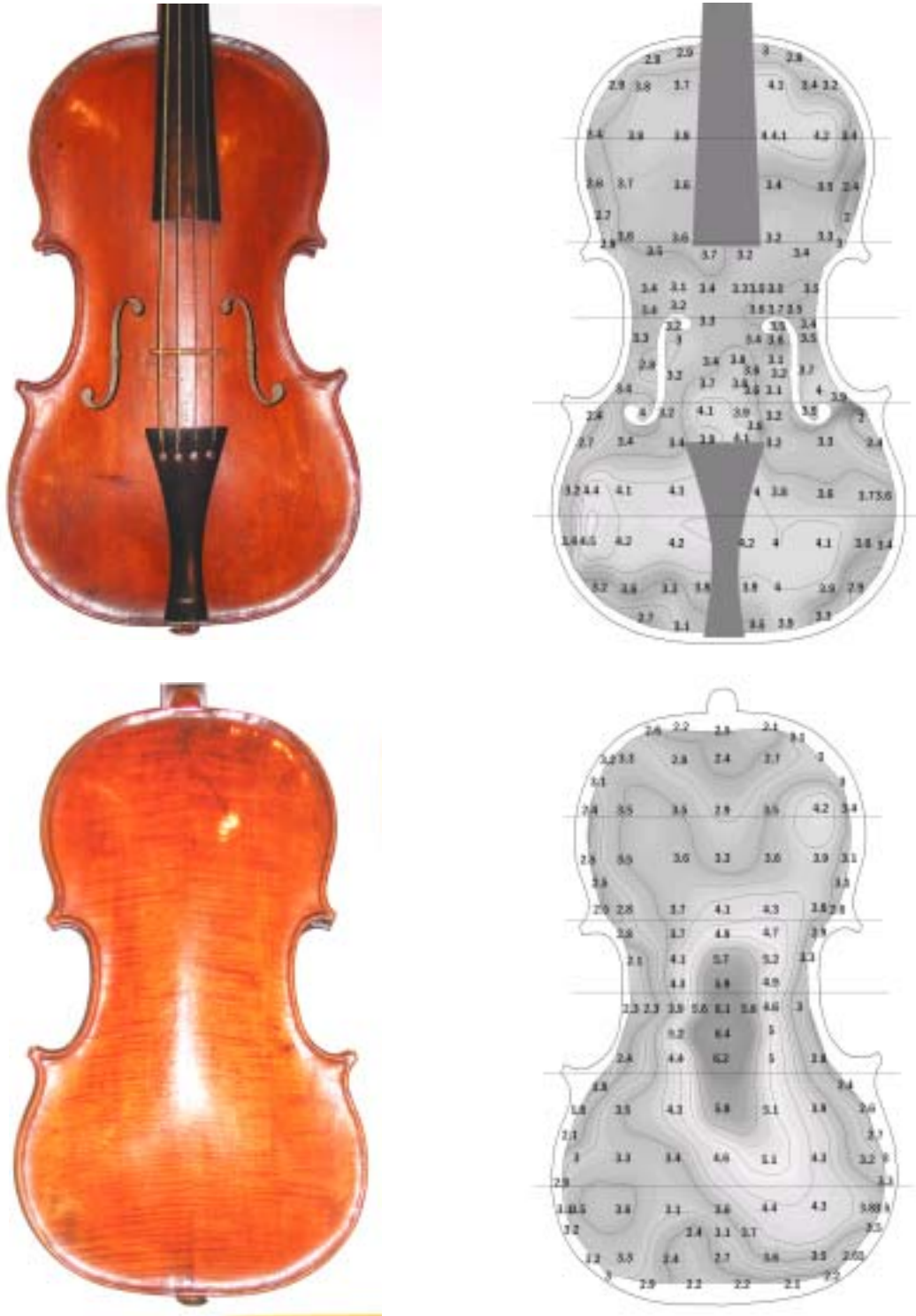
Figure 3. Photos and thickness graduation maps of tenor viola by Andrea Guarneri, 1664, Cremona. Thickness is given in millimeters (0.25 mm contour interval). Dimensions: Body 482 mm, Upper bouts 242.0 mm, Middle bouts 166.6 mm, Lower bouts 280.4 mm, Arching: top 22 mm, back, 20.5 mm, ff-hole spacing 60 mm, Rib height 40.5-44.5 mm, Weight 829 g. Horizontal lines show approximate positions of CT scan cross-profiles shown in Figure 4.
