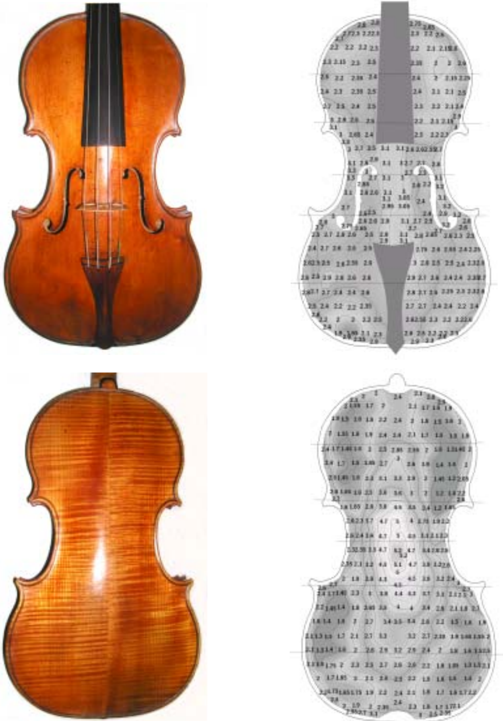
Figure 1. Photos and thickness graduation maps of violin by Nicolò Amati, 1628, Cremona. Thickness is given in millimeters (0.25 mm contour interval). Dimensions: Body 352 mm, Upper bouts 165.5 mm, Middle bouts 106.5 mm, Lower bouts 205 mm, Arching: top 18.0 mm, back 16.7 mm; ff-hole spacing 36.5 mm, Rib thickness 0.9-1.05 mm, Weight 381 g. Horizontal lines show approximate positions of CT scan cross-profiles shown in Figure 2.
