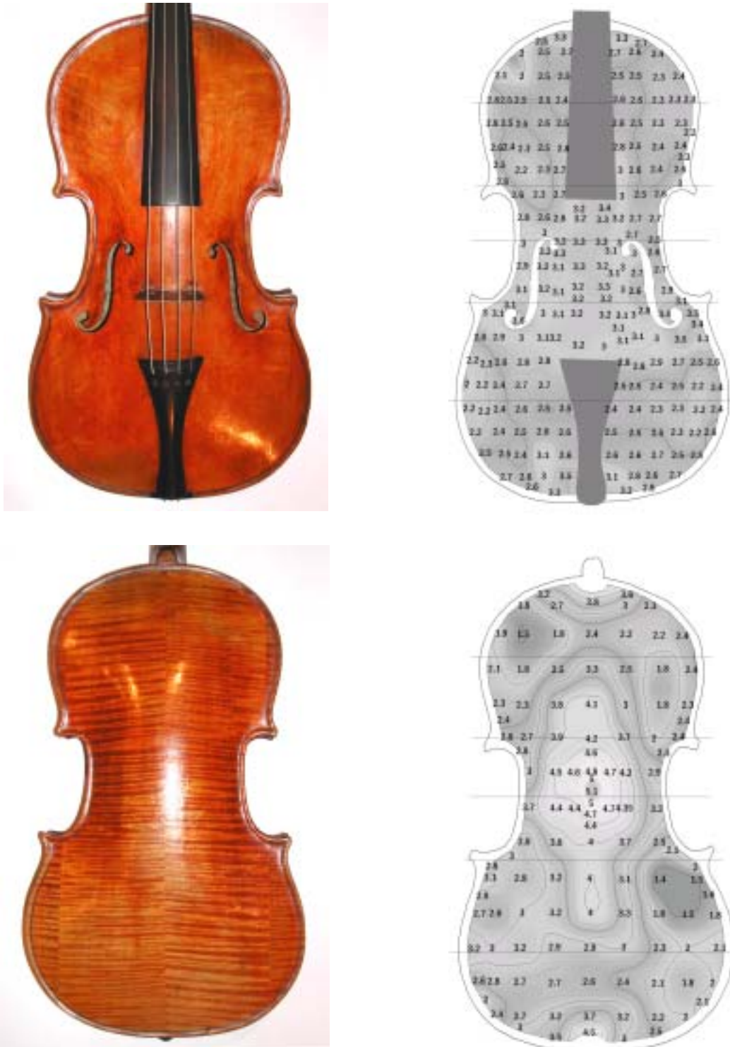
Figure 5. Photos and thickness graduation maps of viola by Nicola Bergonzi, 1781, Cremona. Thickness is given in millimeters (0.25 mm contour interval). Dimensions: Body 410 mm, Upper bouts 196.2 mm, Middle bouts 133.1 mm, Lower bouts 238.9 mm, Arching: top 18.2 mm, back 21.9 mm, ff-hole spacing 61.8 mm, Rib height 31.1-32.8 mm, Rib thickness 0.9-1.2 mm, Weight 561 g. Horizontal lines show approximate positions of CT scan cross-profiles shown in Figure 6.
