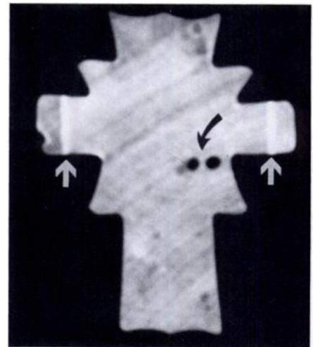
Figure 7. Transaxial CT scan obtained through the scroll of a 1730 Domenico Montagnana cello. Note the hyperattenuating glue lines (straight arrows) from previous repair and wormholes (curved arrow) caused by infestation from the larvae of the beetle, *A domesticum*.
