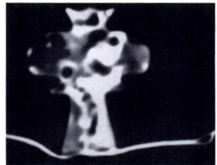
Figure 8. Transaxial CT scan obtained through the scroll of a solo-quality violin. Note the extensive repair with hyperattenuating filler material and associated wormhole damage. The massive extent of repair was not suspected before this CT scan.
