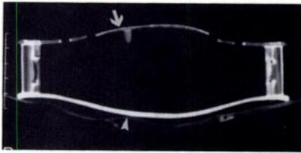
**Figure 9.** Transaxial CT scan obtained through the two "f" holes of a Stradivarius violin at the level of the corner blocks. The front plate is anterior (arrow), and the back plate is posterior (arrowhead).
