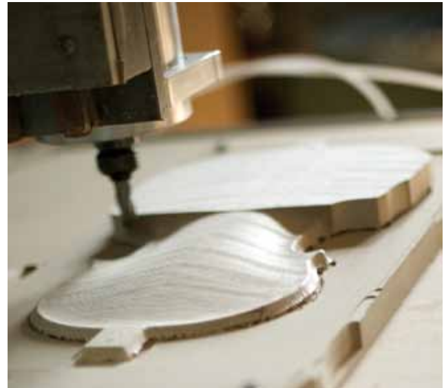
Figure 13 CNC machine cutting replica violin shape
