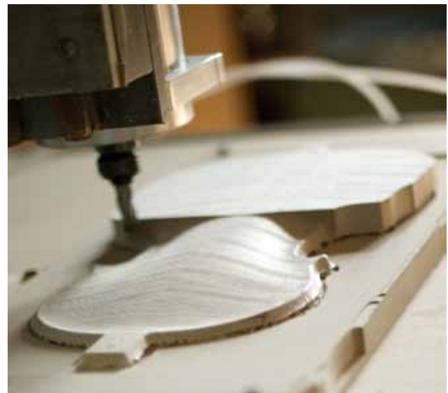
Figure 13 CNC machine cutting replica violin shape
